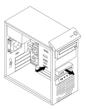
Figure 25. Removing the card reader
